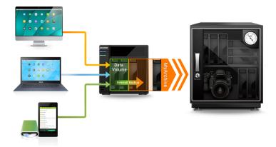
Using the internal backup function allows users to completely utilize the SATA interface's 6Gbps high speed transfers to backup data to MyArchive hard disks. No matter if it's confidential data storage or the archiving of video recording files, all can be scheduled to be backed up to MyArchive hard disks and then transferred to a secure location for safekeeping, meeting the goals of limitless expansion and off-site backup.
